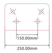
4. Remove the turnstile and use a electric drill to drill holes according to the marks.
